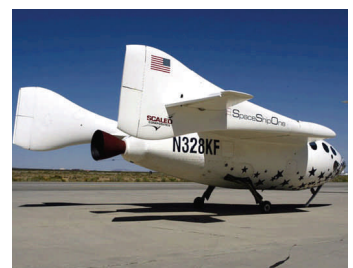
SpaceShipOne has a Hybrid rocket motor.
